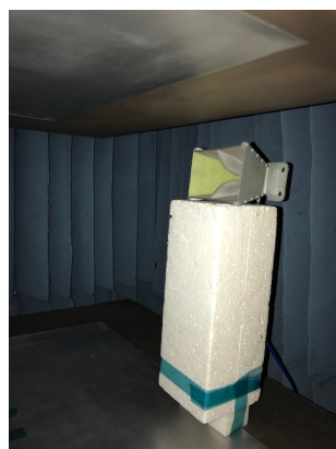
Figure 3.12. Rectangular Feed Horn
